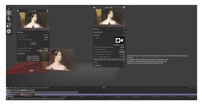
The rotational tracker delay would typically be used in complex gimbal systems - for example, a cable-suspended camera system where the camera is controlled by the gimbal that surrounds it, meaning that both the camera and the cable system are located on two different tracking systems.
